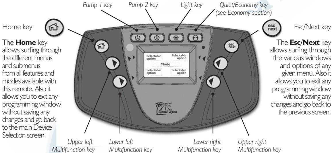
The **Home** key allows surfing through the different menus and submenus from all features and modes available with this remote. Also it allows you to exit any programming window without saving any changes and go back to the main Device Selection screen.
