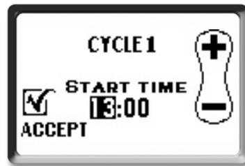
Use the same procedure to set filter cycle duration in hours. If the operation has been successful the display will revert to main Spa Setup window.
